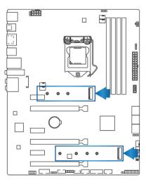
8. Insert the Sabrent ROCKET Q NVMe M.2 SSD device pin-side first into the M.2 slot as is illustrated below.
