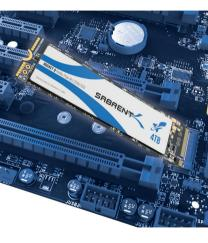
9. Fasten the opposite end of the Sabrent ROCKET Q NVMe M.2 SSD to the motherboard with the necessary screw or hardware, as is illustrated below.
